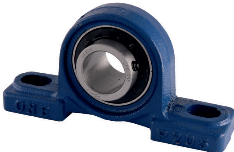
Pillow block bearing with a sealed deep groove ball bearing. The tight fit of the shaft is ensured by grub screws.
