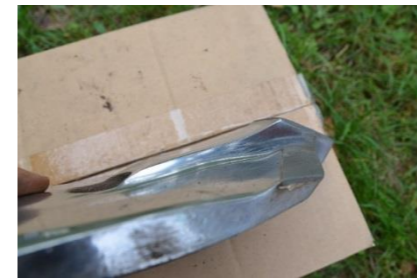
After about 255 hectares, the first abrasion was clearly visible. The edges of the front tip were already ground and there were slight extractions on top of the point. The loss of weight was about 420 g which was nearly 13% of the total mass.
