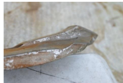
At the end of the year, the points had worked an area of about 360 hectares. While the „F16“ showed almost no further abrasion, the „standard tip was worn out to the half way point of the reinforcement. The loss of weight of the “F16” was about 510 g which was nearly 16.3% of the total mass. The “standard” point had lost around 950 g. That is almost 43% of its total mass. We decided not to use this point any further, because it had some beginning cracks which would have caused it to break soon after.
