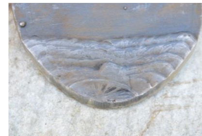
At the end of the year, the points had worked an area of about 360 hectares. While the „F16“ showed almost no further abrasion, the „standard tip was worn out to the half way point of the reinforcement. The loss of weight of the “F16” was about 510 g which was nearly 16.3% of the total mass. The “standard” point had lost around 950 g. That is almost 43% of its total mass. We decided not to use this point any further, because it had some beginning cracks which would have caused it to break soon after.
