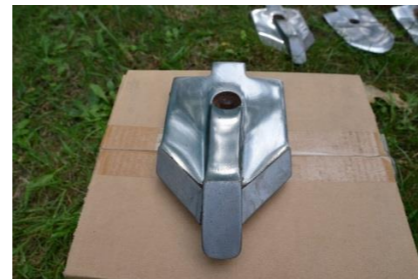
After about 255 hectares, the first abrasion was clearly visible. The edges of the front tip were already ground and there were slight extractions on top of the point. The loss of weight was about 420 g which was nearly 13% of the total mass.
